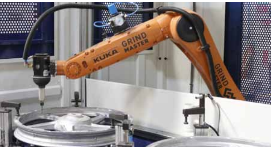
Robotic Fetting Automation
