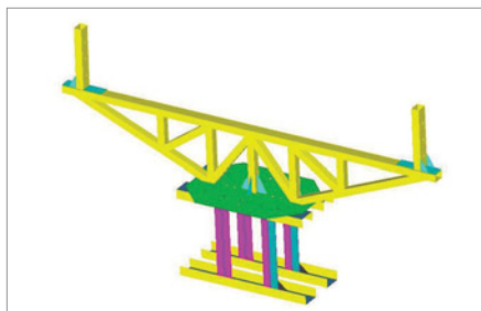
Fixture design for LED board testing on vibration shaker
