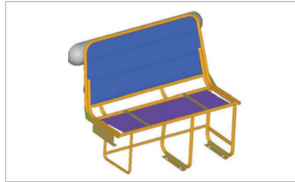
Seat Strength test as per AIS-023
