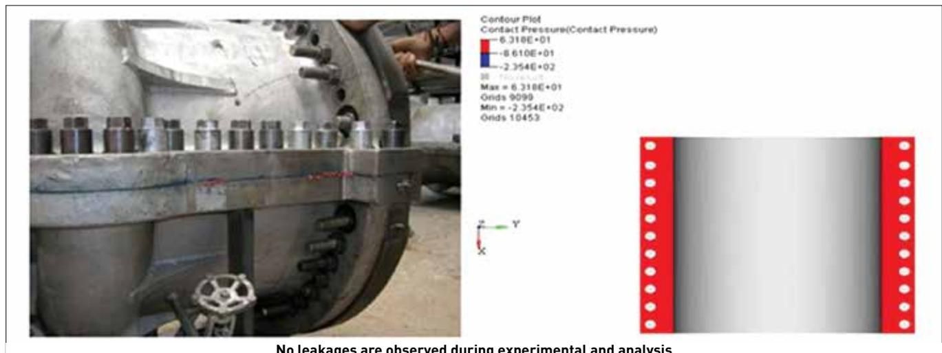
solved further to obtain the reaction forces. The validation is done by taking into consideration a single stage (1st stage) and applying the boundary conditions using ALTAIR HYPERWORKS .High pressure casing of a steam turbine is meshed with Hexa mesh to obtain accurate results.
