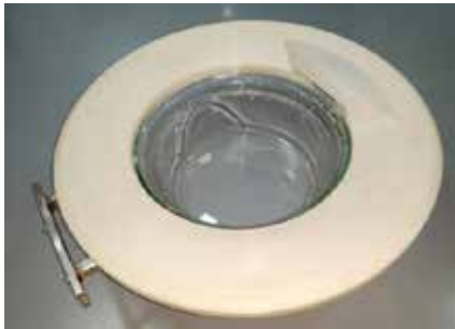
Door assembly 3D printed in ABS Material
