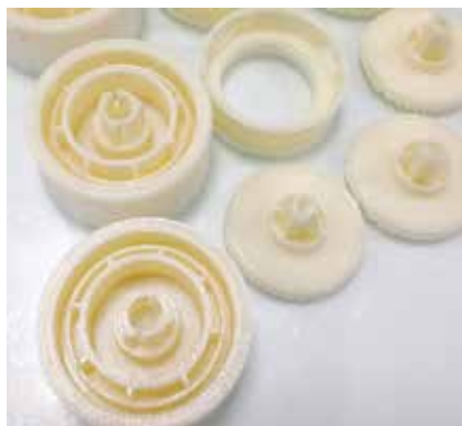
Knob assembly 3D printed in ABS Material
