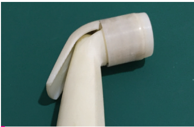
A prototype water spray nozzle 3D Printed in ABS material to validate the nozzle size and flow capacity to withstand the speed of water.
