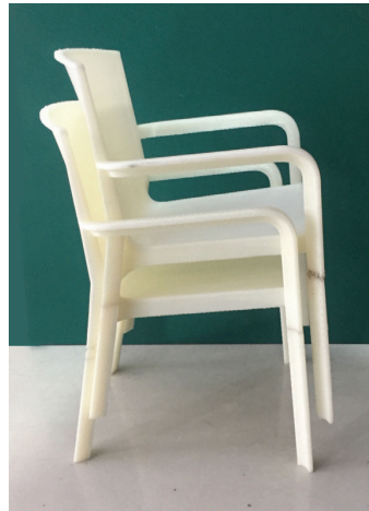
These stacking monobloc chair models were 3D printed in ABS material to check the viability of the design.
