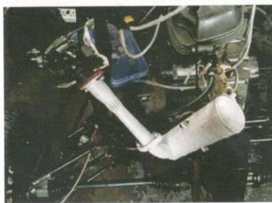
Air-intake prototype inserted into vehicle to test the form
